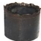
1-3/4" Coil Tubing 0.120" wall thickness RCT-0875-300 cut @ 10,000 psi
