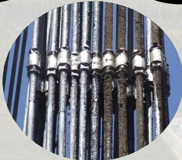
Rods pulled before the installation of a downhole unit.
