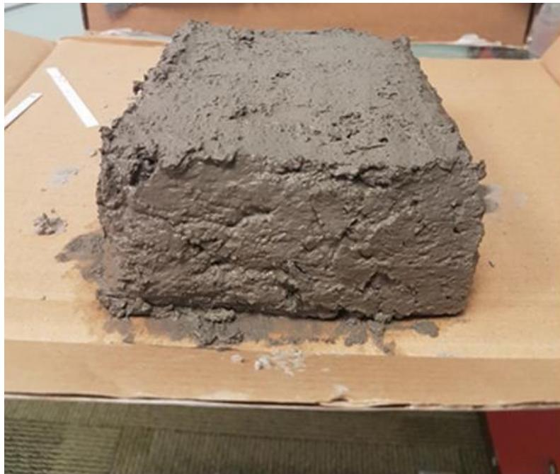
The new DAK-1 technology, through a three-dimensional polymeric network, efficiently encapsulates the free fluid, converting small particles of water into the dispersed phase, complying with the EPA 9095B standard..
